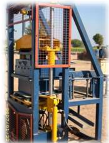
Fig. 7: Semi-automatic block casting machine
